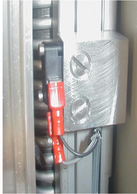
Interior detail, showing part of the spring mechanism and the adjustable end switch for stroke length
